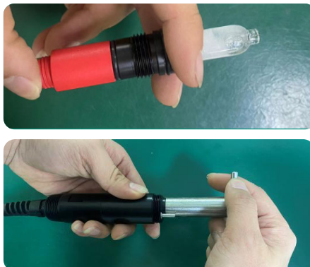
Figure 4-5 Installing the New Electrode
