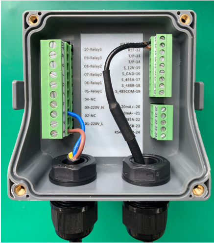
Figure 2-1 Wiring Diagram of Analog Electrode
