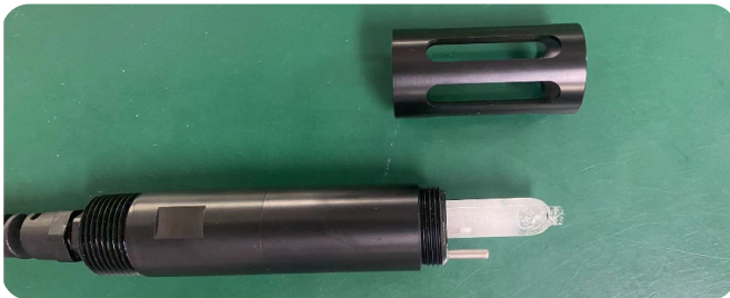
Figure 4-1 ORP Electrode Protective Cover Disassembly Diagram
