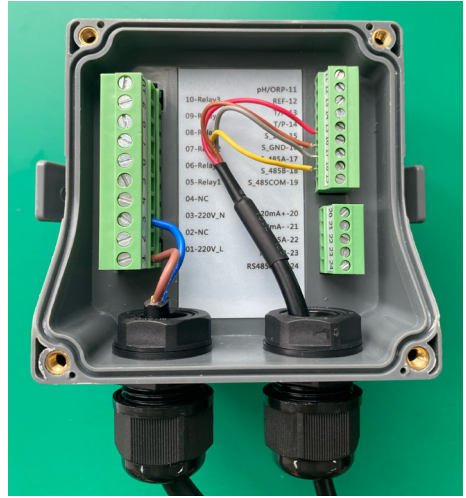
Figure 2-2 Wiring Diagram of Digital Sensor
