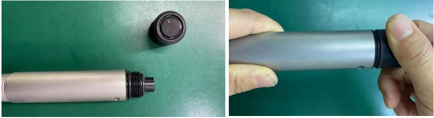
Figure 3-2 Dissolved oxygen membrane cap installation diagram
